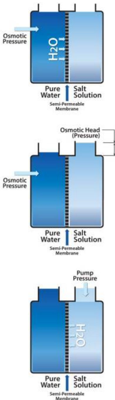
RO and DI filters use different physical reactions to clean water. Reverse Osmosis (RO) is often used to partially clean-up tap water to make it roughly 90% to 99% pure. Deionization (DI) filters exchange positive hydrogen and negative hydroxyl molecules for positive and negative contaminant molecules in water. DI filtering and other processes are sometimes referred to as “water polishing.”
